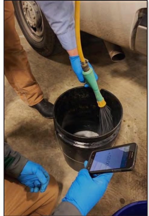
**Figure 1.** Catch test performed using a pre-marked five gallon bucket. Be sure to maintain constant pressure, measure time precisely, and check multiple times to ensure accurate catch test results. Photo credit to Josh Landreth - Ace of Blades, LLC.
