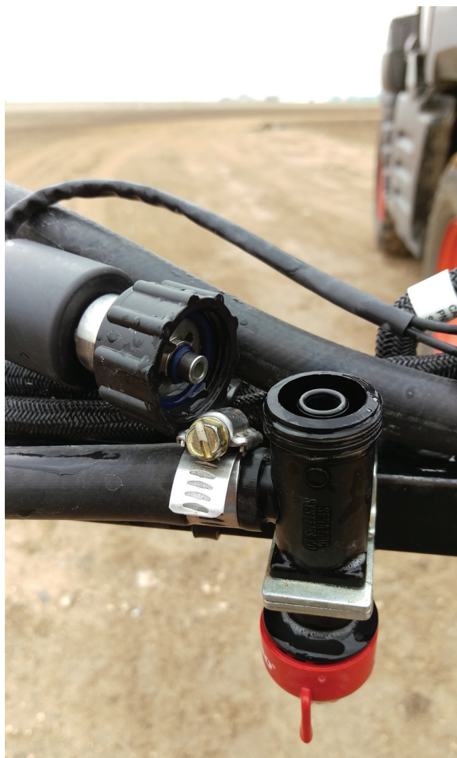
Figure 1. Solenoid valve equipped on PWM sprayer.
